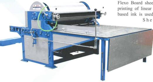
Flexo Board sheet printer is useful for printing of linear paper & board. Water based ink is used for printing. Printing Sheets can be used
